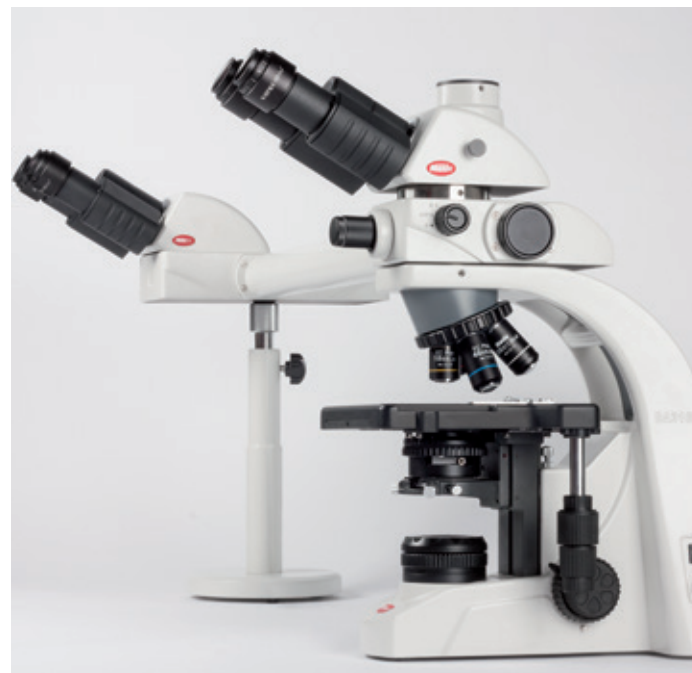
MULTI-VIEWING DEVICE · SIDE-BY-SIDE
