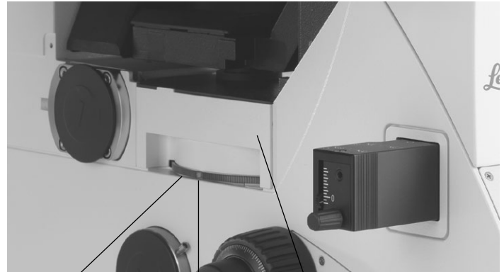
Knurled ring for setting the filter cube Color mark Cover
