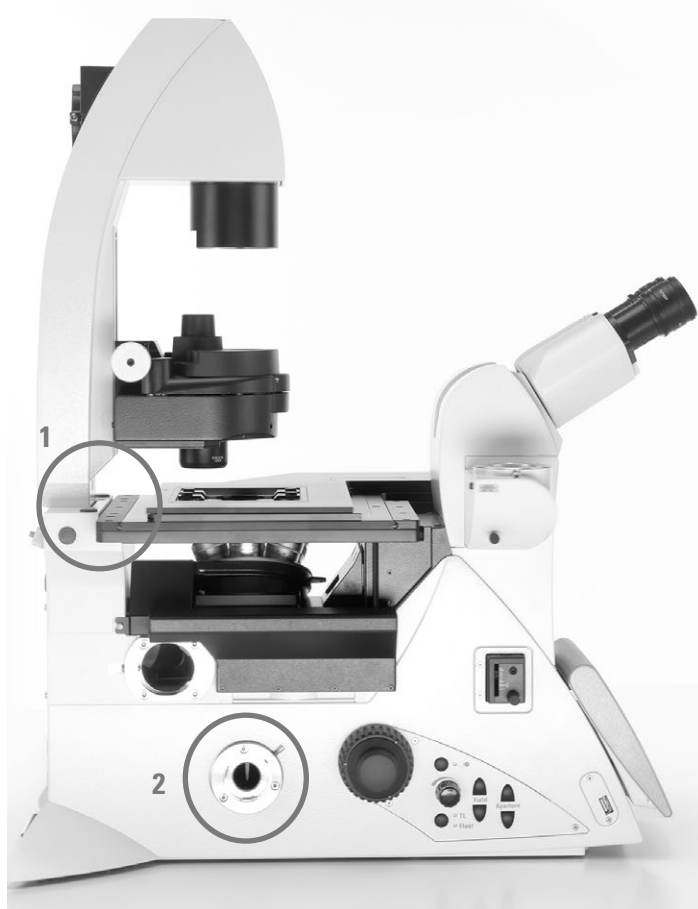
Interlock switch (1) and (2)
