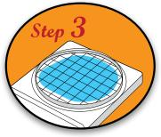
Specimen diffuses automatically into the plate, transforming the dry medium to gel.
