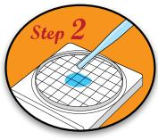
Drop 1ml of specimen (dilute if necessary) in the middle of dry sheet.
