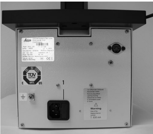
Fig. 24 Rear view of the Leica DM IL LED Leica DM IL LED Fluo and DM IL M LED equivalent 1 Power supply connection
