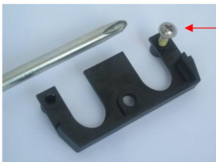
Cut the thread with the screw
