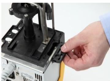
The pump connection set can only be mounted on one side of the control head. (see illustration).
