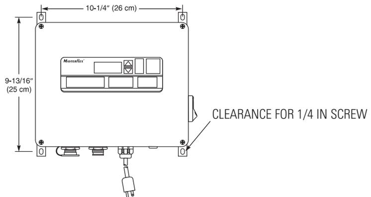
**Figure 2-2.** Control Box Mounting Dimensions 77111-10, 77111-15, 77111-40 and 77111-47.
