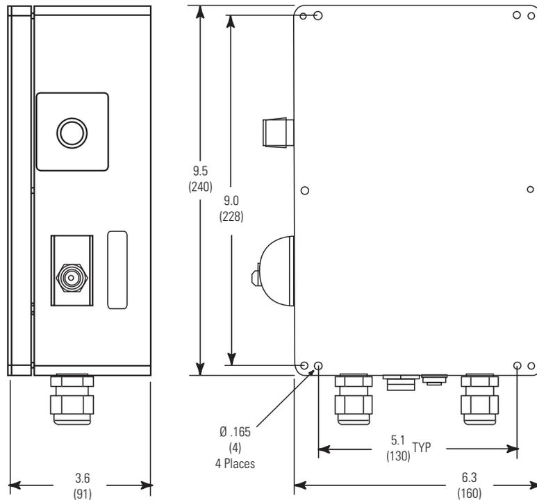
**Figure 2-4.** Control Box Mounting Dimensions 77111-67 (230V).
