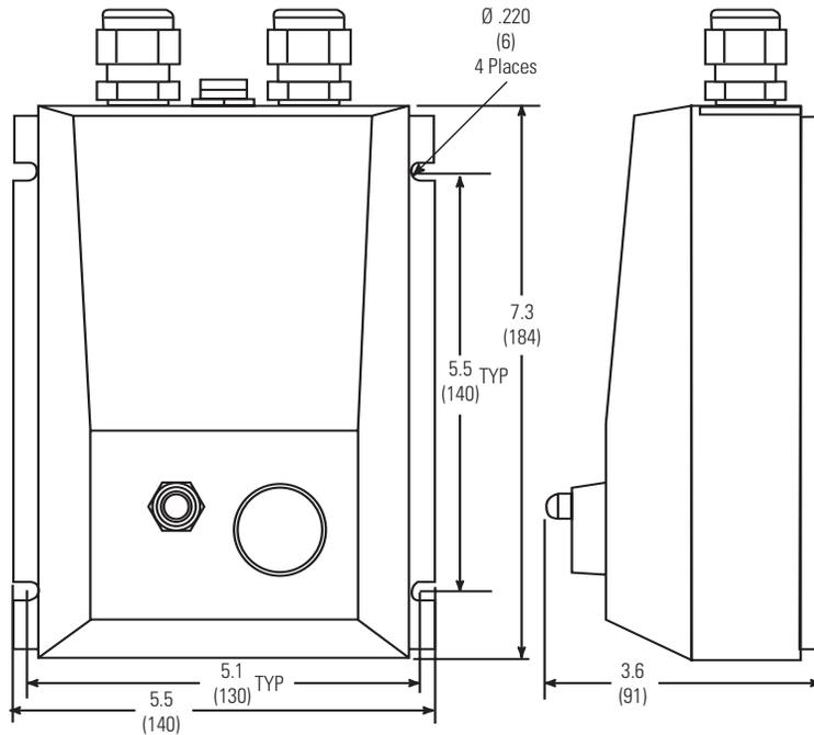
**Figure 2-3.** Control Box Mounting Dimensions 77111-60 (115V).
