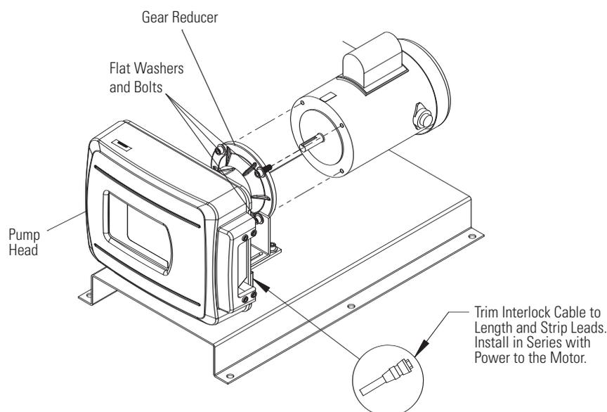
Figure 2-7. Motor Mounting IEC-72 71-14F130 Motor Frame
