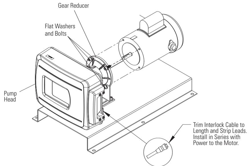
Figure 2-6. Motor Mounting NEMA TYPE 56C Motor Frame
