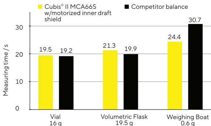
**Figure 7:** Measurement times in drafty conditions test results.
