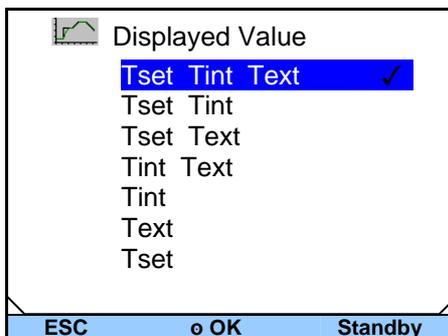
With display measurements you can define which temperature values are to be graphically displayed. In the menu all possible combinations are offered.
