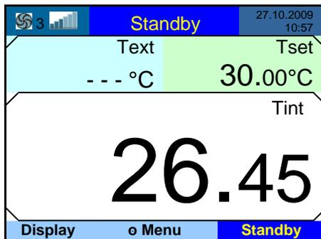
If standby is activated ( $\Rightarrow$  7.4.4), "Standby" appears in the expanded status display. The "Standby" soft-key function is highlighted in a different colour.
