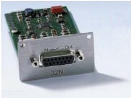
Contact module (order no. LRZ 915) with 15-pole SUB-D socket. Range of functions as LRZ 914, but with three relay contact outputs (changeover, max. 30 V/0.2 A) and three binary inputs for control via external voltage-free contacts.
