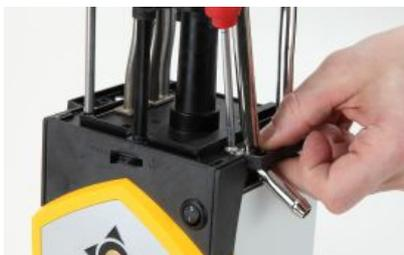
The cooling coil can only be mounted on one side of the control head. This is located on the side with the mains switch (refer to illustration).
