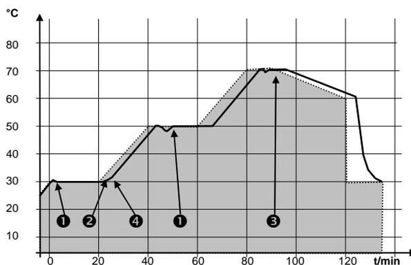
Example of the effect of the tolerance input with external bath control:
