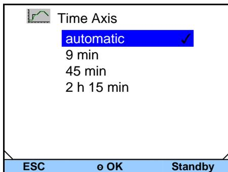
With "Time Axis" you can define the temporal range over which the measurements are to be displayed.
