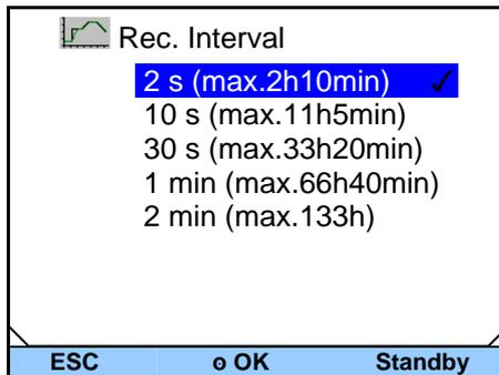
With "Rec. Interval" you can define the time interval at which the temperature measurements are to be recorded. The values in brackets give the maximum recording time. In the menu five possibilities are offered.
