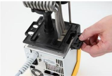
The pump connection set can only be mounted on one side of the control head. With the control head turned round and the mains cable pointing to the user this is then on the right (refer to illustration).
