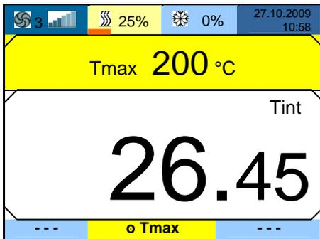
Check or set the overtemperature switch-off point with the key
