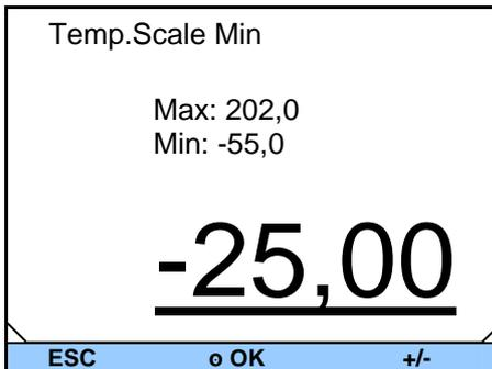
When "Temp.Scale Max" or "Temp.Scale Min" (as in the illustrated example) has been selected, the entry window appears.
