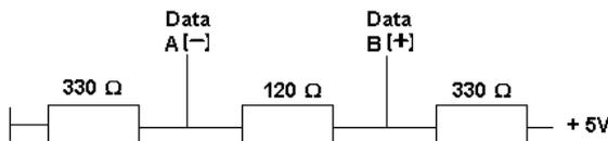
Generally, this terminating network is integrated on the PC plug-in card (RS 485).
