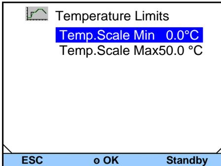
With "Temperature Limits" you can manually input the temperature limits for the graphical display.
