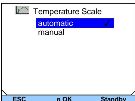
With "Temperature Scale" you can define the scaling of the y axis (temperature value).
