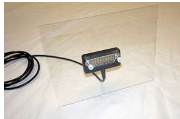
Figure 5. The wireless alpha ionizer components.
