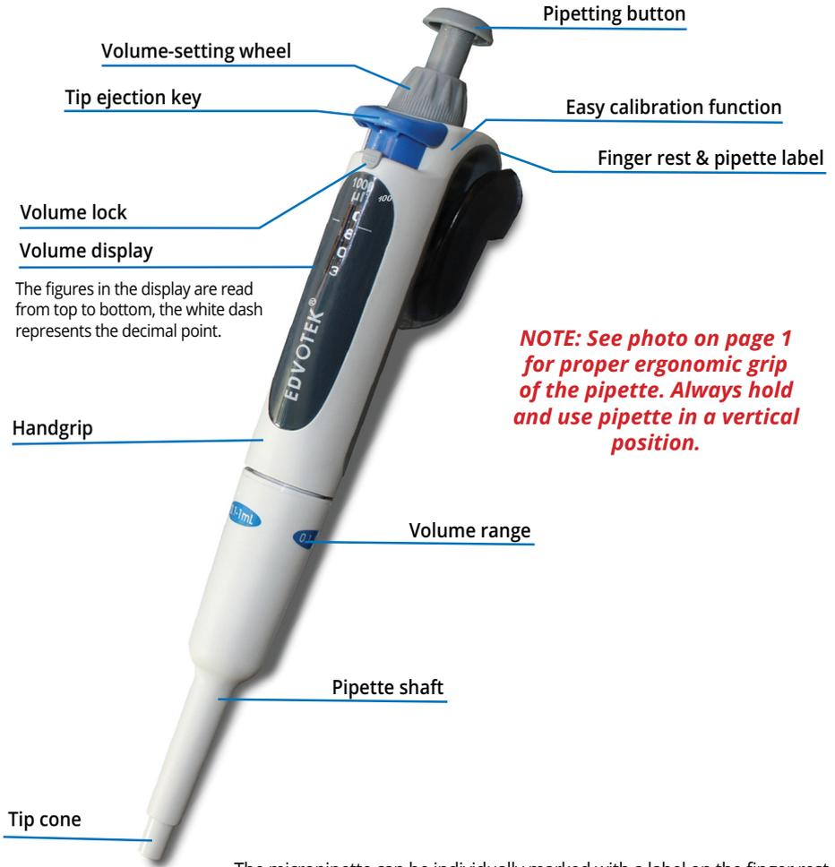
**NOTE: See photo on page 1 for proper ergonomic grip of the pipette. Always hold and use pipette in a vertical position.**
