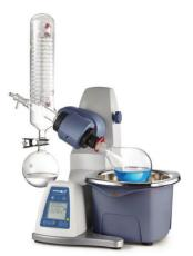
Boil-dry protection, unit automatically powers off if heating without water/oil in the heating bath
