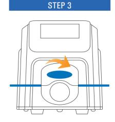
Turn the pump head handle counterclockwise to raise the upper section of the pump head Place the tube into the opening, ensuring that the tube is:
