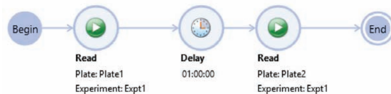
Figure 2. Workflow setup in SoftMax Pro Software. The initial read at time zero is followed by a one-hour delay (incubation), and then the plate is read again. The instrument is set to 37°C prior to start of the workflow.
