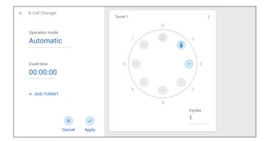
Touch and the instrument will automatically set the instrument to zero absorbance and 100% transmittance. Once the calibration has been performed the turret will automatically measure each sample.
