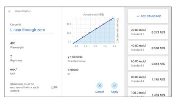
Specific points can be selected on the graph by touching the graph, a sliding cursor will appear. It is possible to move the cursor by dragging left or right.
