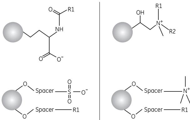
**Fig 3.16.** Design principles of CDM libraries. Multimodal cation exchangers (left) and multimodal anion exchangers (right) are illustrated.
