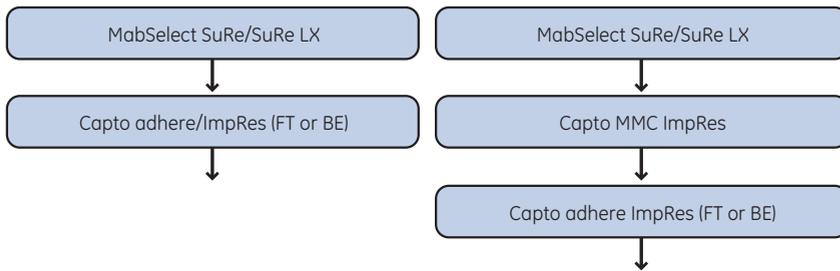
**Fig A3.1.** Strategy for use of multimodal media in two- and three-step processes for MAb purification. FT = flowthrough; BE = bind/elute.
