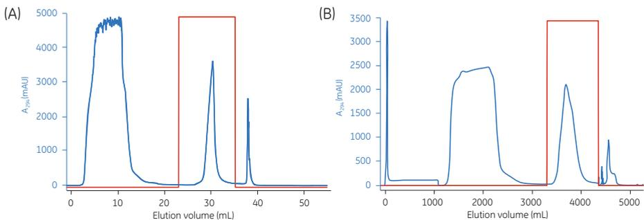
**Fig 4.48.** Straightforward scale-up from A) Tricorn 5/100 to B) AxiChrom 50 (100 times). In both cases the purification factor was 4 and the recovery was 93%.
