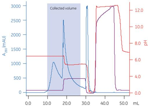
**Fig 4.24.** Chromatogram from the column verification. Blue: Absorbance at 280 nm. Red: pH. Purple: Conductivity (mS/cm).
