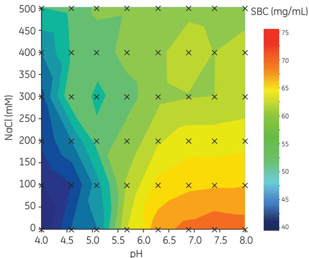
Fig 4.30. Contour map showing screening of SBC for Capto adhere ImpRes.
