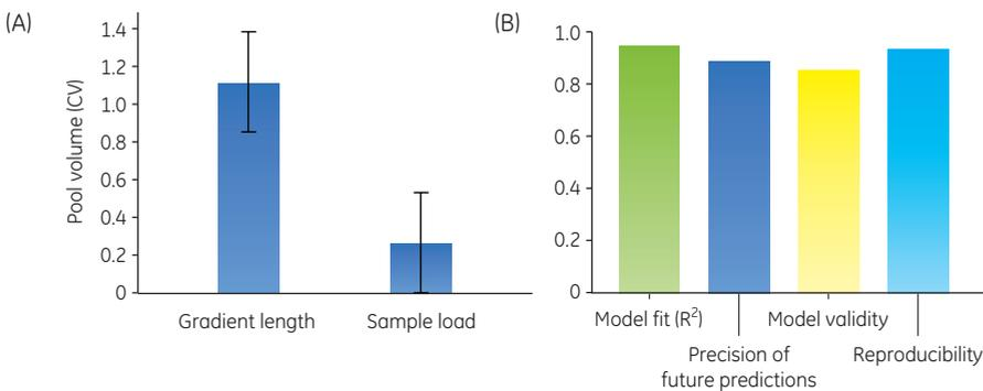
**Fig 4.55.** (A) Coefficient plot showing factors affecting pool volume. (B) Summary plot showing different model characteristics for the response pool volume.
