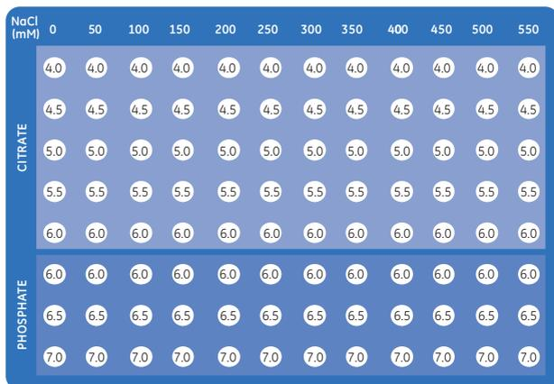
**Fig 4.15.** Plate layout of the selective elution study.
