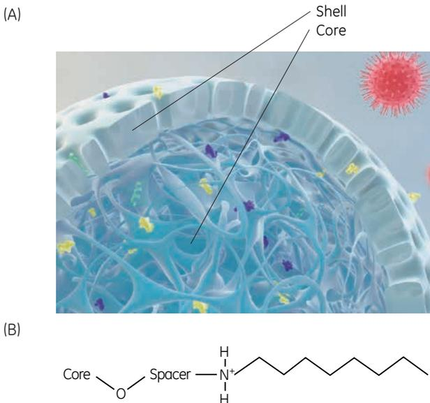
**Fig 2.2.** (A) Schematic representation of the principle for Capto Core 700 showing a bead with the inactive porous shell and the ligand-activated core. Small proteins and contaminants (colored green, yellow, and purple) penetrate the core while target viruses (red) and larger proteins are excluded from the medium and are collected in the flowthrough. (B) The immobilized ligand in the core.
