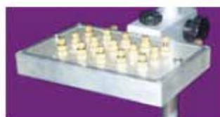
Multi-Needle manifold with individually controlled flow
