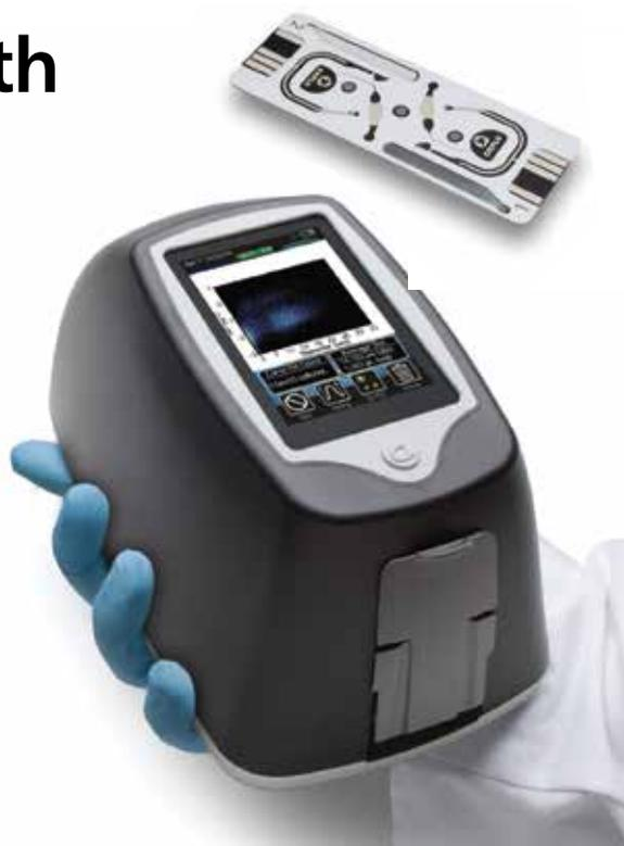
precisely counts and sizes particles (Coulter Principle) and exactly measures fluidic volume. The entire test is performed on-cassette, so no fluid enters the system, obviating the need for time-consuming cleaning, disinfecting, and shutdown procedures.
