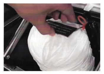
Note the cartridge's position should be 3-4 inches BELOW top of the tracks. Remove the yellow ribbon and cardboard.
