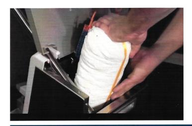
Push downward and forward (keeping the cartridge at a 90 degree angle), allowing the clips to enter easily in the slots. Note the use of both hands to ensure all clips enter the tracks.
