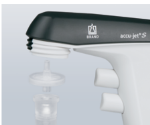
Membrane filter and check valve prevent liquid penetration and over-aspirating liquid
