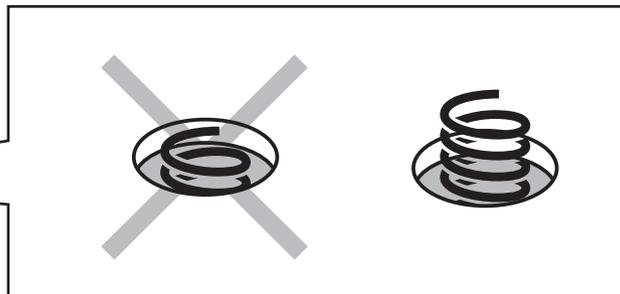
Check the grounding spring. Make sure that the grounding spring juts slightly out of the hole.
