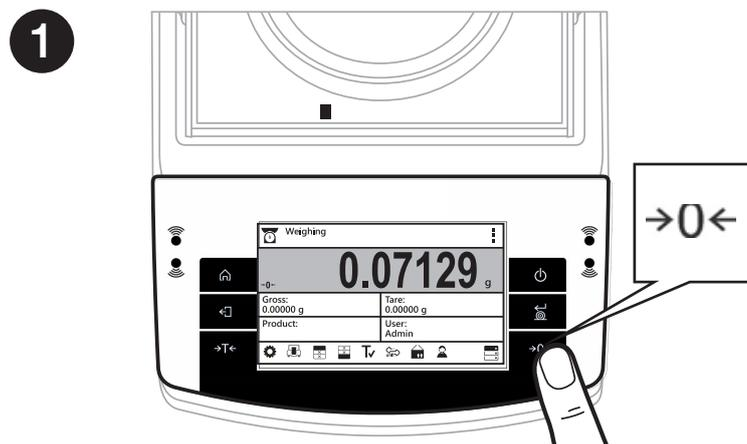
Unload the weighing pan and press "Zeroing" button.
