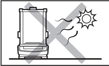
Place the balance away from heat sources. Avoid exposing the balance to the sunlight.
