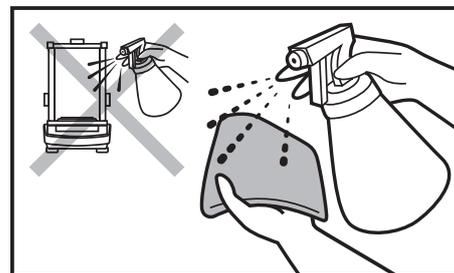
Apply the cleanser onto the cloth first. Avoid applying the cleanser directly onto the device.
