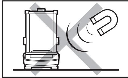
Avoid exposing the balance to a magnetic field. Do not weigh magnetic substances.
