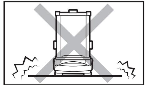
Do not place the balance on an unstable ground exposed to shocks and vibrations.
