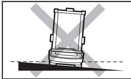
Make sure that the balance is placed on an even surface.
