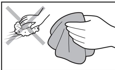
Use soft cloths made of microfiber, natural fiber or man-made fiber. Avoid using abrasive cloths or cloths that might scratch the surface.
