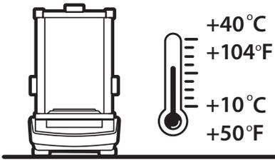
Operate the device in a room where the temperature ranges between 10–40 °C (50–104 °F) and where the relative humidity is below 80%.
