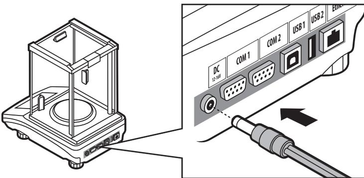
Connect the power adapter to DC connector.
