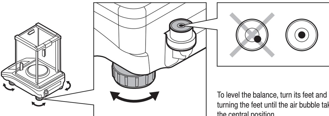
To level the balance, turn its feet and keep turning the feet until the air bubble takes the central position.
