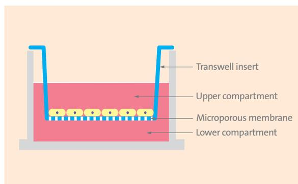
The unique, self-centered hanging design of Transwell inserts prevents medium wicking between the insert and outer well. The design also permits access to the lower compartment through windows in the insert wall, as well as undamaged co-culturing of cells in the lower compartment.
