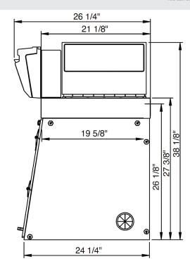
Please add 6" between the last filter and the ceiling to allow for good air recirculaton and to replace filters easily.
