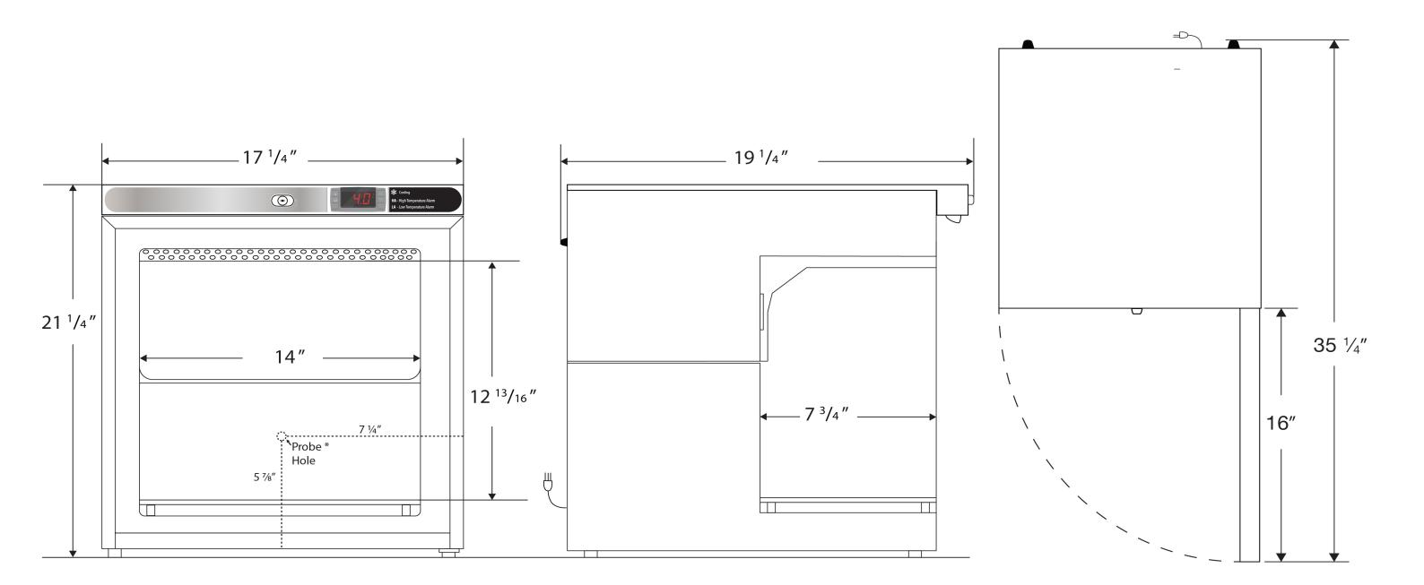
Note: This unit must have 4" clearance on sides and back for adequate ventilation
