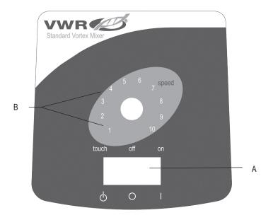
The front panel of the Standard Vortex Mixer contains all the switches and control knob needed to operate the unit.
