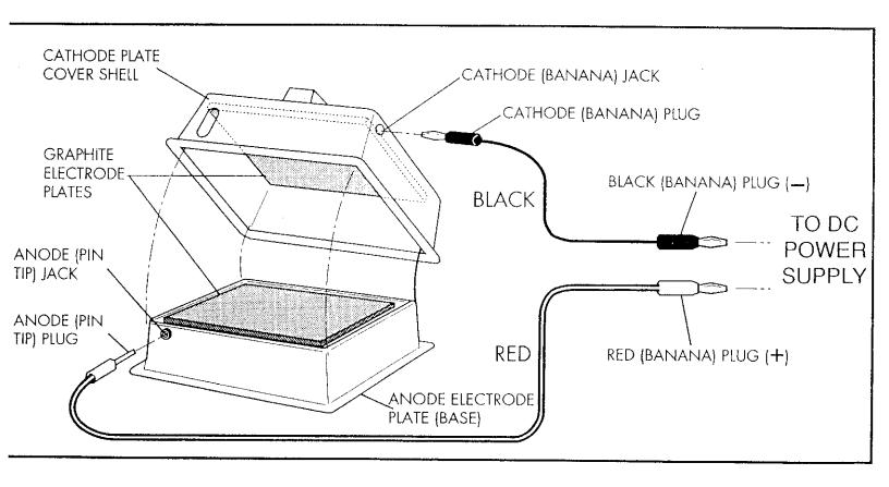
Figure 2 - Building A Trans-Unit Stack
