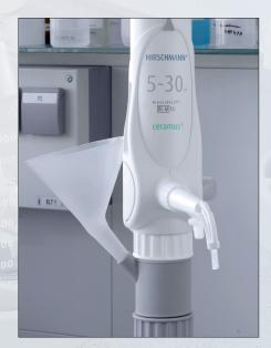
Adapter with NS 12/21 filling tube for funnel
