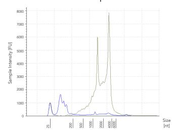
Small RNA (<200 nt) is separated from large RNA (>200 nt) using the RNA Clean & Concentrator™ MagBead. Size was analyzed using the Agilent 2200 TapeStation® system.
