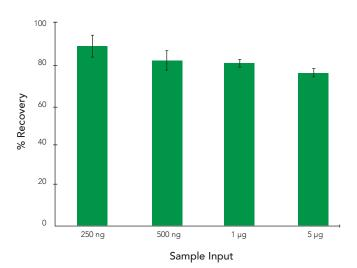
Select-a-Size DNA Clean & Concentrator® MagBead shows efficient recovery at different concentrations. DNA recovery (≥80%) is consistent from low to high amounts of genomic DNA input (n=3).
