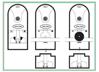
In preparing the unit for performing experiments, make sure that the paper tape is running under the carbon wheel.
