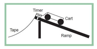
Next try mounting a piece of timer tape to a cart. You may need about eight feet for this. Mount the timer as shown and set up the ramp. Allow the cart to travel down the ramp and roll across the table while pulling the tape. You should notice from the marks on the strip that the dots started off close together. This coincides with the actions of the cart starting from a resting state, accelerating and then losing momentum and once again slowing back down.
