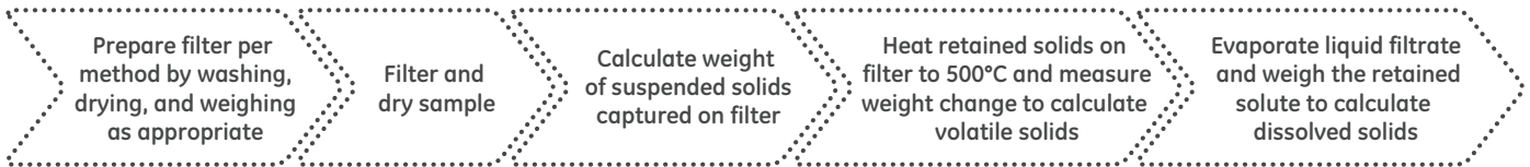
Fig 1. Total solids analysis workflow using filtration-based methods.
