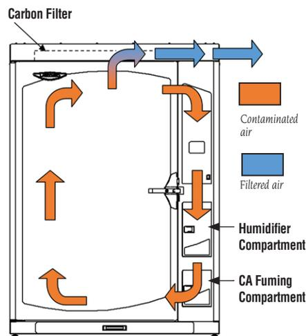
During the humidifying or fuming cycle, air is recirculated within the chamber. The recirculation blower pulls air from the top of the chamber and directs it to the bottom of the chamber. During the exhaust or purge cycle, the exhaust blower draws air from inside the chamber through a pre-filter and carbon filter located above the top of the chamber. The exhaust blower then directs the filtered air back into the room via slot openings located on the right side rear.
