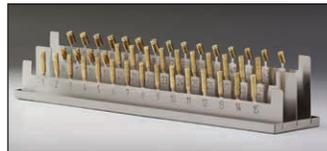
**10014-344 Casing Holder Kit.** Provides 45 numbered standoffs for upside down casing placement. For casings .32 caliber or larger. Shipping weight 10 lbs. (5 kg)
