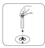
Remove vial from the sample chamber.
