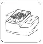
Seal the vials in the preheated thermoreactor for 120 minutes at 150°C
