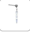
Add 6 - 7 g soda lime powder into the absorption tubes.
