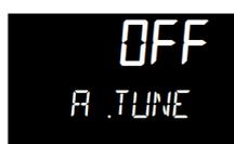
4. To enable the auto-tune, set the A.TUNE parameter to ON by using DOWN
