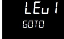
When Level 1 is selected the display reverts to the HOME display. A passcode is not required when moving from a higher level to a lower level.
