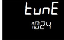
The auto tune is completed when the regular display of the measured temperature is shown and the process is allowed to control at the target set point using the new control terms.
