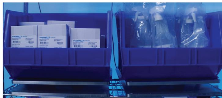
**Smart shelves:** Rather than having stockroom personnel deliver materials to individual labs, smart shelves are installed in storage rooms located near labs. They incorporate sensors that can detect when materials stored in them are getting low and, through linkages with inventory management tools, initiate timely restocking — a simple yet valuable way to reduce stock-outs and prevent overordering of materials.
