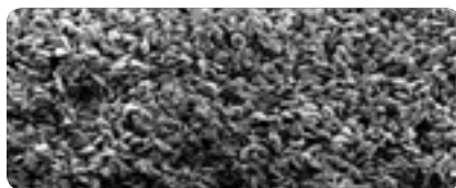
B. High-performance silica HPTLC plate
