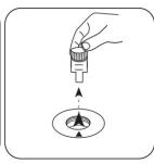
Remove the vial from the sample chamber.
