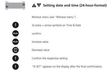
The instrument returns to the measurement mode.
