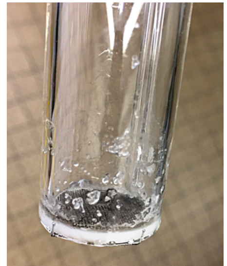
Fig. 10. Crystals from Reagent M in the cathodic compartment. Generator electrode can sometimes turn black due to impurities in Reagent M.
