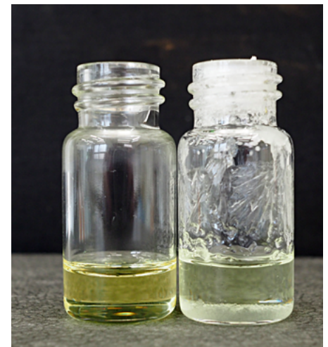
Fig.12. Hydranal-Coulomat AG (left) and Reagent M (right) after four days in open vials.
