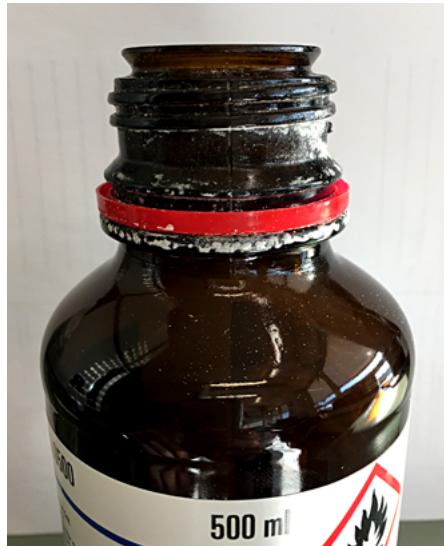
Fig. 9. Bottle neck of Reagent M after five titration cell fillings. Reagent M crystallizes very fast and contaminates the bottle neck.
