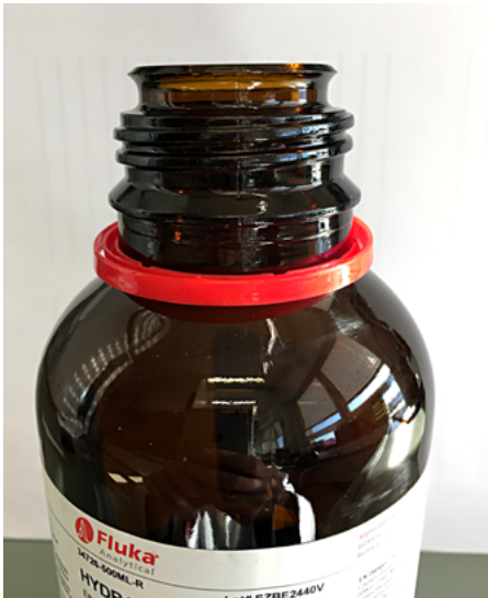
Fig. 8. Hydranal-Coulomat AG bottle neck after five titration cell fillings. Crystallization is suppressed.
