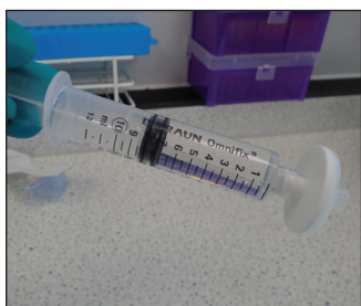
7. The syringe filter is flipped over and the outlet side is connected to a new 10 mL syringe, filled with PBS.
