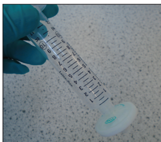
2. Remove the syringe plunger and attached the 10 mL syringe to the filter inlet.
