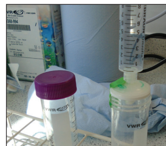
3. Place on top of an open 50 mL collection tube and secure with tape.
