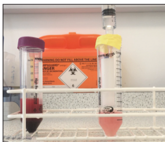
8. The filter with the syringe is placed on a new collecting tube, and the PBS is pushed through the filter.
