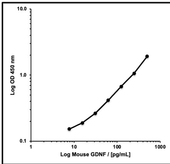
In the above example graph, GDNF standards were run in triplicates using the assay diluent provided in this kit. The TMB reaction was stopped after 25 minutes.
