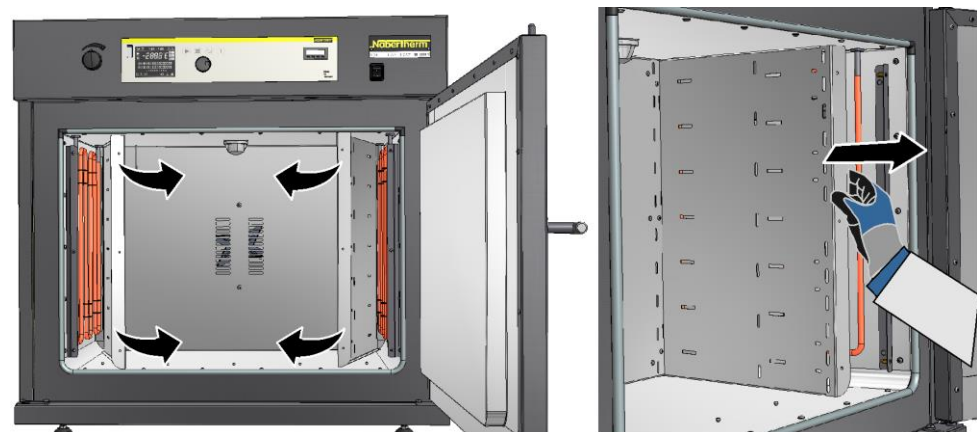
Fig. 49: Removing the side walls from the oven (similar to picture)
