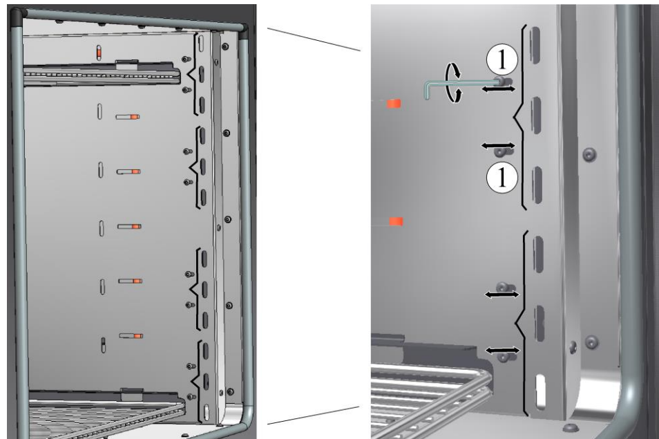
Fig. 24: Adjusting the individual baffles (similar to picture)
