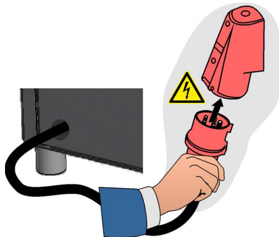
Fig. 16: Furnace from 3.600 W (CEE plug) (similar to picture)
