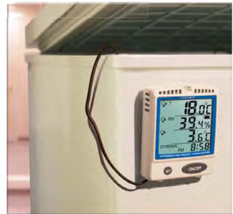
Thin cable is makes it easy for refrigerator door to close and seal
