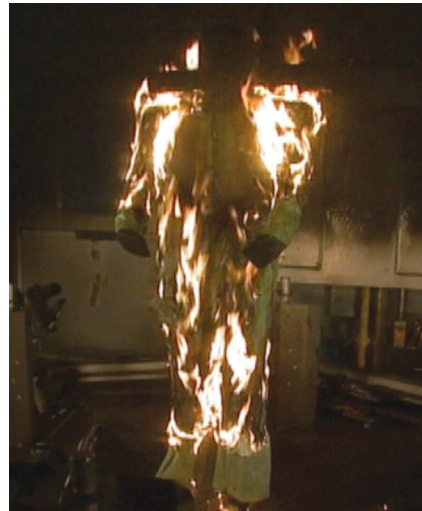
This standard (non-flame resistant) chemical protective garment ignites and melts onto the manikin during a similar flame exposure, resulting in significantly higher levels of predicted burn injury. (Image 3 seconds after flame source removed.)
