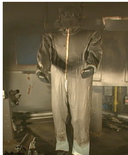
The Tychem® 6000 FR garment does not continue to burn after the flame exposure—maintaining a protective barrier to minimize burn injuries. (Image 3 seconds after flame source removed.)
