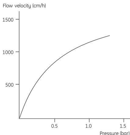
**Fig 3.** Pressure/flow velocity curve for Sepharose 4 Fast Flow in XK 50/30, bed height 15 cm (a) and BP 113, bed height 5 cm (b); mobile phase H<sub>2</sub>O.
