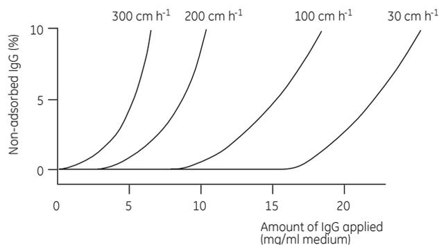
**Fig 4.** One example of how the capacity for human IgG depends on the flow velocity with nProtein A Sepharose 4 Fast Flow. The non-adsorbed IgG (%) was measured as a function of the amount applied to the column at 4 different flow velocities, 300, 200, 100, and 30 cm/h. Concentration of the applied sample: 0.33 mg IgG/ml. Column: 0.5 × 5 cm (i.d. × h). Buffer system: 0.1 M Na<sub>2</sub>HPO<sub>4</sub>, pH 7.0.
