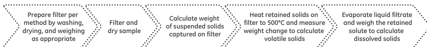
Fig 1. Total solids analysis workflow using filtration-based methods.
