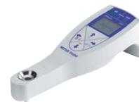
The Refracto 30PX has an optical glass prism held by a stainless steel ring. The Refracto 30GS has a sapphire prism held by a ring of hard gold-plated brass. Sapphire has a higher refractive index and better thermal conductivity than glass. For this reason, the Refracto 30GS has an extended measuring range and registers sample temperature more quickly.
