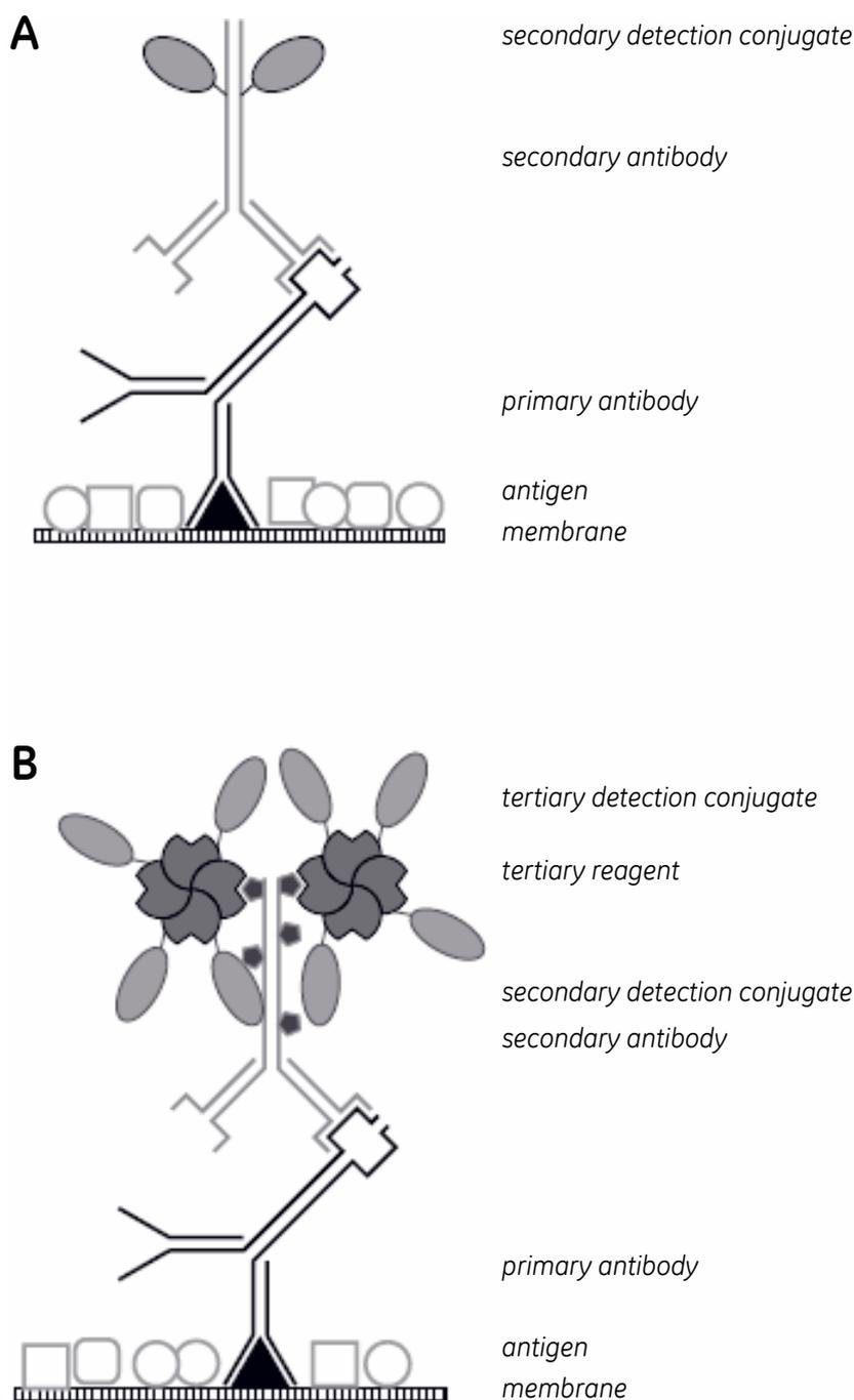
**Fig 1-1.** Indirect detection of blotted antigens.
