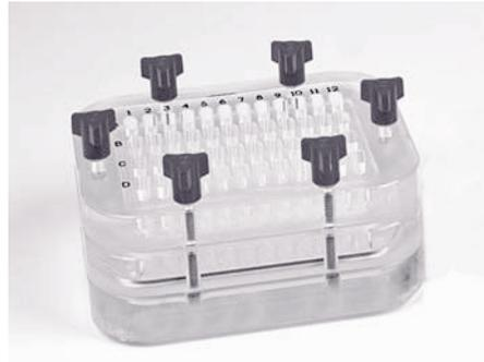
**Fig 1-3.** Slot Blot Manifold with 48 sample filtration slots.
