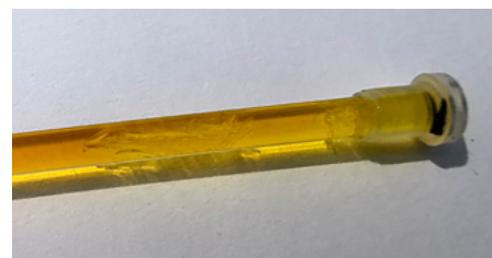
Fig. 2. Example of dosing tube contaminated with crystals.
