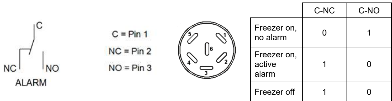
Figure 22: Zero-voltage contacts circuit diagram and pin allocation of DIN socket
