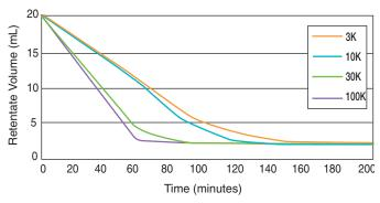
Protein solutions were processed in each of the Macrosep Advance devices. Average time (minutes) is plotted against mL of remaining product to be filtered using a swinging bucket rotor at 5,000 g. Solutions are 3K: Protamine Sulfate, 0.1% in 1X PBS; 10K: Cytochrome C, 0.025% in 1X PBS; 30K: IgG, 0.1% in 1X PBS; and 100K: Apoferritin, 0.1% in 1X PBS.
