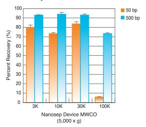
A 500  $\mu$ L sample of a 100  $\mu$ g/mL DNA fragment solution containing 50 and 500 bp double-stranded DNA fragments was centrifuged at 5,000 x g in Nanosep devices to a final volume of 50  $\mu$ L. Recovered samples were quantified using absorbance at 260 nm. The 100K device was able to differentiate between the sizes of the DNA fragments.
