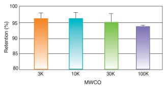
Proteins solutions were processed in each of the Macrosep Advance devices. Average percent retention using a swinging bucket rotor at 5,000 g is displayed for each MWCO. Solutions were 3K: Protamine Sulfate, 0.1% 1X PBS; 10K: Cytochrome C, 0.025% in 1X PBS; 30K: IgG, 0.1% in 1X PBS; and 100K: Apoferritin, 0.1% in 1X PBS.
