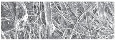
DUPONT™ TYYEK® IS MADE WITH A UNIQUE FLASH-SPINNING PROCESS THAT CREATES A TORTUOUS PATH FOR PARTICLES.
