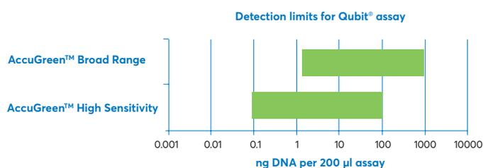
FIGURE 1: Chart comparing the linear detection ranges for AccuGreen™ kits for Qubit® fluorometer.
