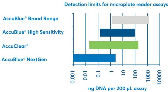
FIGURE 4: Chart comparing the linear detection ranges for dsDNA quantitation kits for fluorescent microplate reader.
