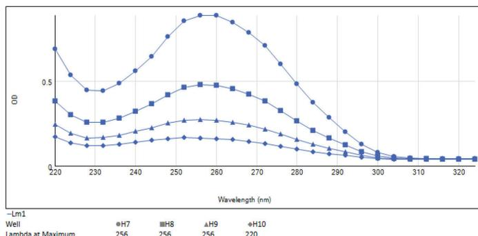
**FIGURE 3:** SoftMax Pro software pre-configured data table. Spectral scans were performed to assess sample purity. Four representative concentrations of DNA were scanned and only a peak at 260nm was identified, indicating pure dsDNA.
