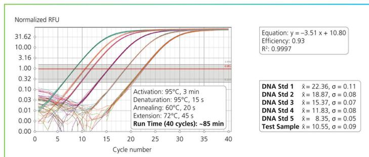
**FIGURE 1: Reliable results across runs.** Pre-diluted 426bp DNA standards were amplified in a typical three-step cycling protocol that completes in approximately 85 minutes. Results show the highly repeatable Cq values obtained across four distinct trials.
