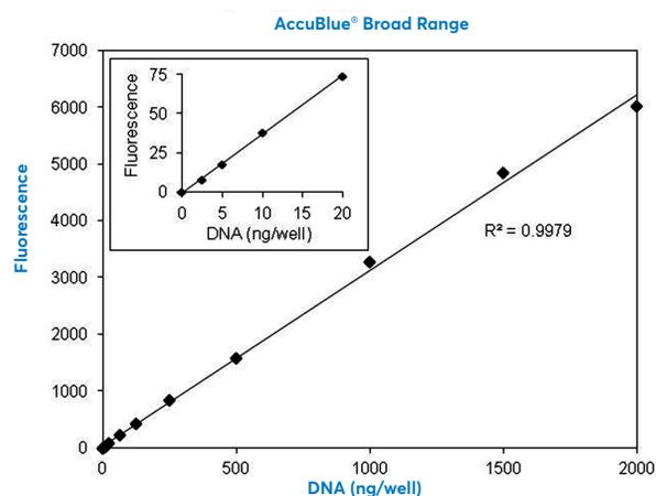
FIGURE 8: Standard curve of calf thymus DNA assayed using AccuBlue® Broad Range Kit and read on a microplate reader (Ex/Em 350/460). Inset shows the lower end of the titration.
