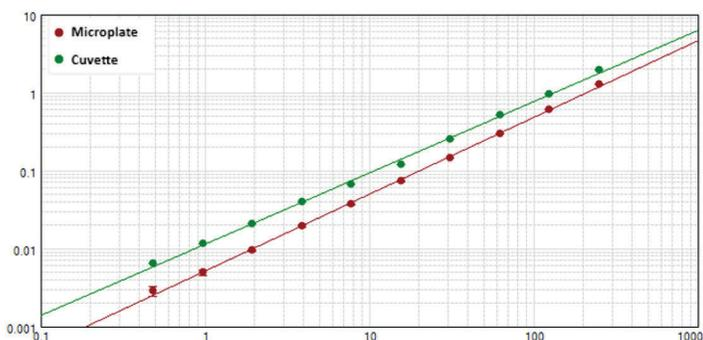
**FIGURE 4:** dsDNA quantitation in a 96-well microplate or cuvette. The dsDNA dilution series was detectable from 250 to 0,50ng/μl in both cuvette and microplate formats. Additionally, both dilution series demonstrated high linearity.
