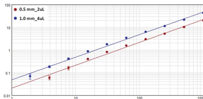
**FIGURE 1:** dsDNA quantitation on the SpectraDrop micro volume microplate. The ABS Plus reader with the SpectraDrop microplate could detect down to 2 and 4 ng/μl of DNA using the 1.0mm (blue) and 0.5mm (red) coverslips respectively.
