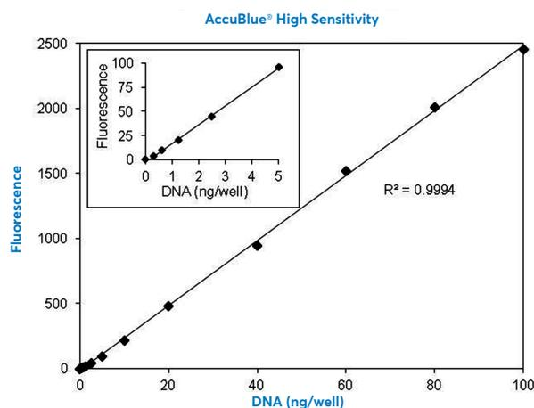
FIGURE 7: Standard curve of calf thymus DNA assayed using the AccuBlue® High Sensitivity kit and read on a microplate reader (Ex/Em 485/530nm). Inset shows the lower end of the titration.
