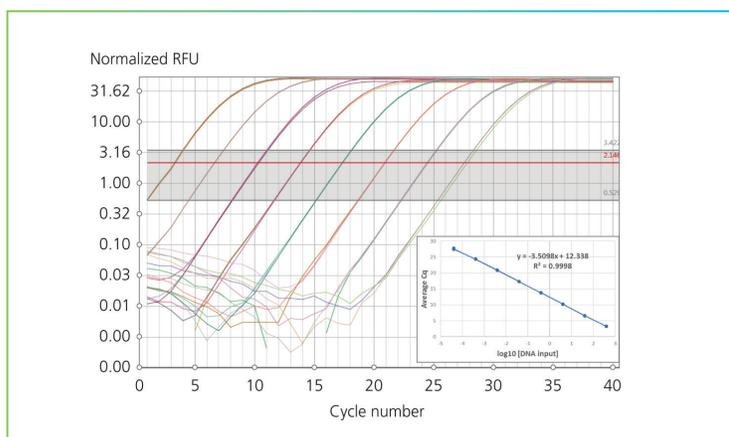
**FIGURE 2: Samples from multiple NGS libraries were pooled into a test sample with average fragment size of 450bp.** A 10-fold dilution series was prepared and assayed on the Q. Analysis of the resulting amplification curves showed high efficiency and sensitivity across an 8 log dynamic range.
