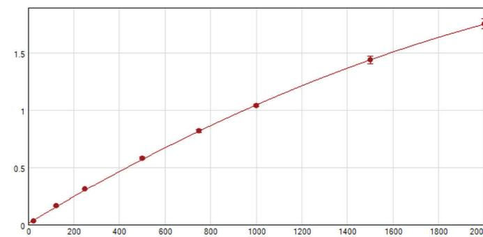
**FIGURE 5:** BCA Assay standard curve. The ABS Plus microplate reader was able to detect the BSA standards from the BCA assay. SoftMax Pro software was used to apply a quadratic curve fit to the data points, and a robust standard curve ( $r^2 = 1,000$ ) was generated.
