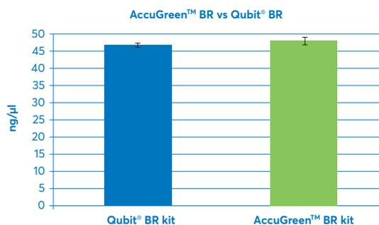
FIGURE 3: A genomic DNA sample was quantified using both the Qubit® BR kit and the AccuGreen™ BR kit using a Qubit® 3 fluorometer. A nearly identical result was obtained with each kit.
