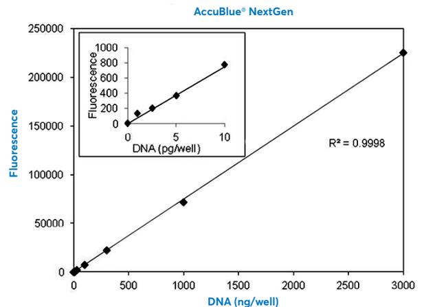
FIGURE 6: Standard curve of calf thymus DNA assayed using the AccuBlue® NextGen kit and read on a microplate reader (Ex/Em 460/507nm). Inset shows the lower end of the titration.
