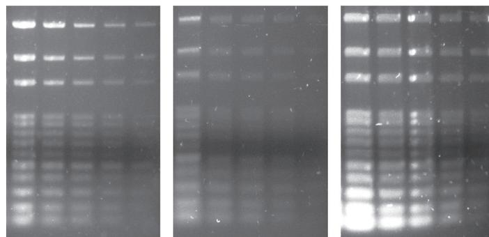
**Comparison of EZ-Vision® Blue Light DNA Dye to GelGreen™ and SYBR® Green I** Two-fold dilution series of identical DNA fragments were electrophoresed in 1% agarose gels. The gels were then stained with EZ-Vision Blue Light (left panel), GelGreen (middle panel) and SYBR Green I (right panel). DNA fragments were visualized using a blue light transilluminator and SYBR Green filter.
