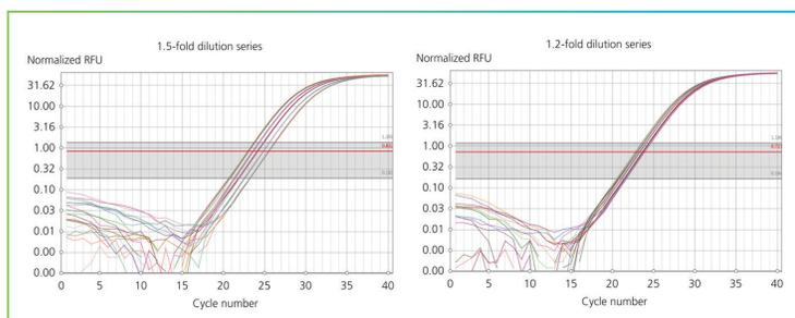
**FIGURE 3: A range of dilution series were prepared from the 426 bp unknown test sample for qPCR analysis on the Q.** Results show the ability of the Q to clearly distinguish samples in both a 1.5-fold and 1.2-fold dilution series.
